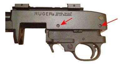
With the barrel and receiver out of the stock as shown on the left, use a punch to remove the trigger assembly by removing the indicated pins. They usually remove best from left to right with the gun in the shooting position.
