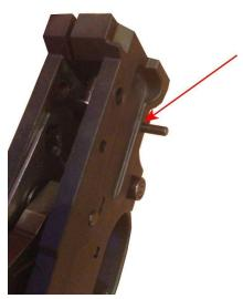
Remove the old Bolt Lock plate and replace with the TANDEMKROSS Guardian Bolt Release Plate. The orientation for the plate can be seen here. The fit can be tight. The plate slides down until just the very end of the plate is out of the housing and the bottom and top holes line up. The bottom pin goes through the oval opening and the top pin goes through the larger "D" shaped cutout.
