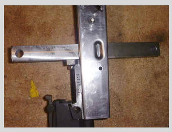
Once the "T" block is adjusted it will be placed inside of the receiver/trunion. Slide the machined bar into the receiver after the "T" block is installed. This is then placed in the shop press with the barrel facing up towards the ram of the press. Support the bar on your press plates or pieces of scrap steel if you don't have the press plates.
