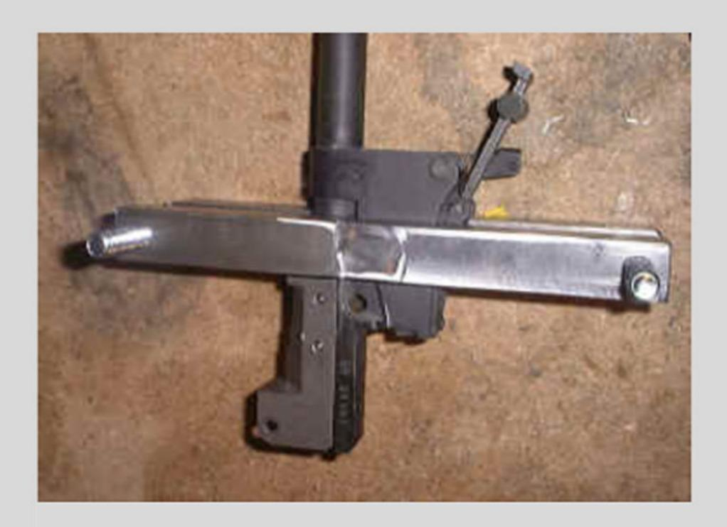
You will need to flip your rear sight forwards to clear the bars. If you don't have press plates or extra metal to lay across your shop press to support the bars so they run horizontally across the base of the shop press you can angle the bars across the base. If you have to angle the bars across the base be careful not to let the sight to hit anything.
