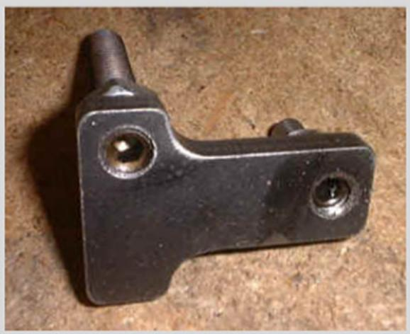
The "T" shaped piece is designed to hit the trunion in three spots. The left side of the "T" hits the rear left portion of the trunion. The short set screw fits into the magazine notch and the long set screw hits on the front area.
