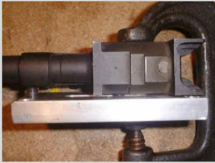
Here you can see the front set screw plus the middle and rear set screws leveling out the trunion on the aluminum plate. The cut-outs in the plate let you use this method with or without rivets installed.
