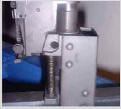
Once the barrel is in place all that's left is to press the pin back into the trunion/barrel assembly. Use the short punch to install the pin.
