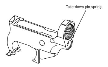
Ensure the weapon is unloaded with the safety engaged! Remove the stock from the rifle, remove the buffer and action spring from the buffer tube, and then remove the buffer tube (receiver extension) from the receiver. When removing the stock and tube from the receiver, use care not to lose the take-down pin spring and detent. For detailed information on removing the stock assembly from the receiver, refer to the firearms manual or the US Army Maintenance Manual TM 9-1005-319-23&P.
