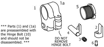
Using a 9/64 Allen Wrench, remove the Hex Screw (6) from the Side Plate Cover (2). Next, remove the Side Plate Cover (2) from the receiver side of the Hinge Assembly (1). With the plate cover removed, separate the Button Spring (3) and Button (4) from the Hinge Assembly (1).
