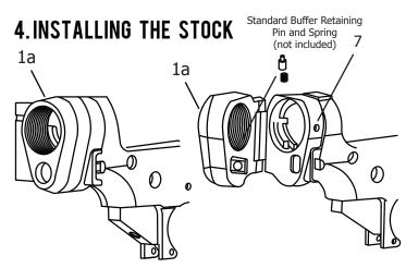
With the folding stock adapter tightly installed on the receiver, using a 3/32 Allen Wrench, tighten Flange Set Screw (7) to secure the Threaded Flange. Make snug but do not over tighten.
