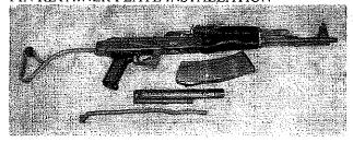
Start with the selector, carrier, bolt, and recoil spring assembly removed from your rifle. Pull the retainer wire (Shepherd's Crook) from the grooves of the trigger and hammer pins, and remove it from your rifle.
