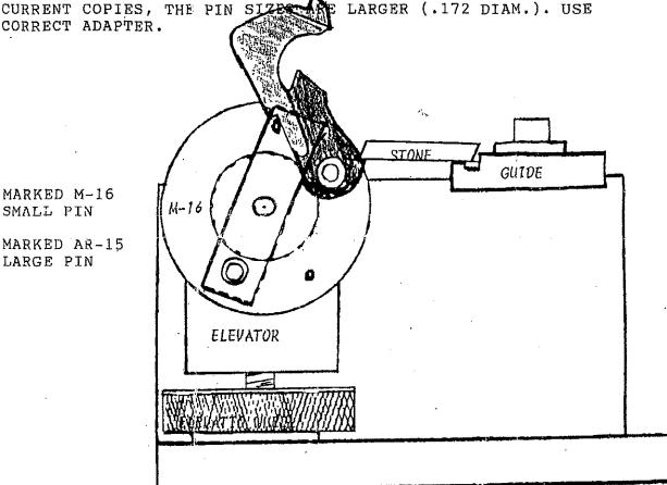
NOTE, LOCATION OF CLAMP ON HAMMER & TRIGGER. RECTANGLE DOTTED LINE REPRESENTS CLAMP.
